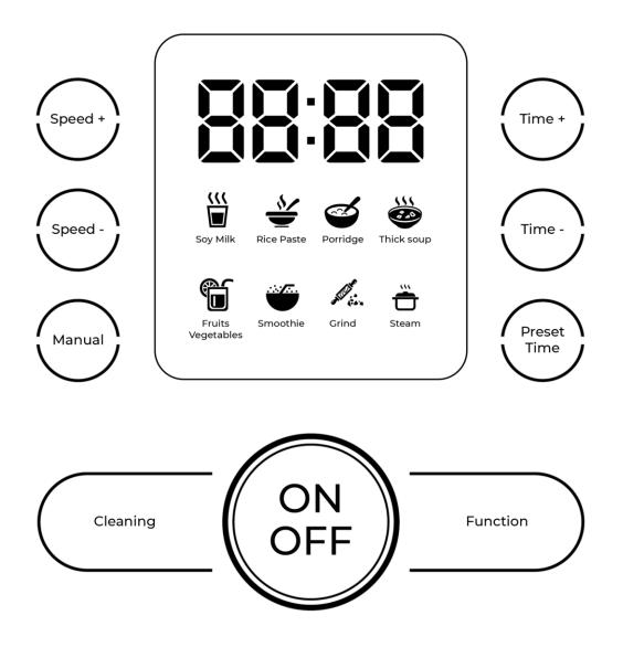
Figure 4 – Device control panel
